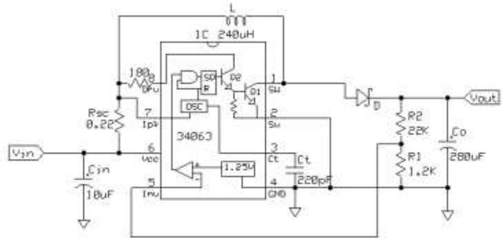
Figure 5 DSU Reconfigured as Boost Mode
