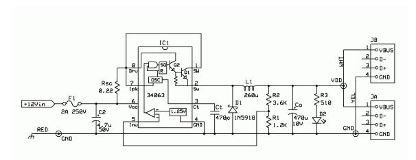
To modify the unit take off the fuse ferule and pry apart the case. Unsolder the fuse spring, the wired-in USB connector (JB) and the one mounted on the circuit board (JA), resistors R1, R2 and R3, and any wires remaining on the board.
