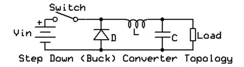
The switch can be turned on and off very rapidly and the ratio of the ON duration to the cycle time will determine the ratio of the average output voltage to the input voltage  $V_{out} = \frac{t_{ON}}{t_{ON}+t_{OFF}}V_{in}$ .
